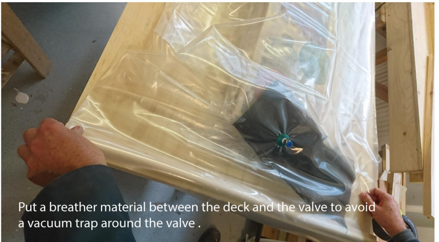
Put a breather material between the deck and the valve to avoid a vacuum trap around the valve .
