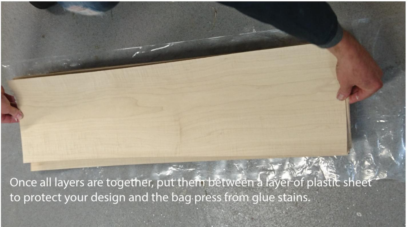
Once all layers are together, put them between a layer of plastic sheet to protect your design and the bag press from glue stains.
