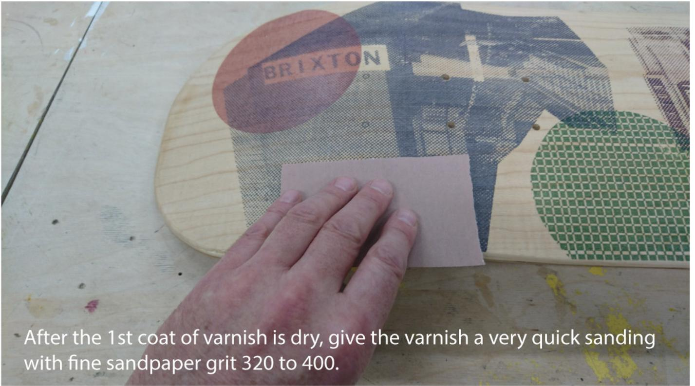
After the 1st coat of varnish is dry, give the varnish a very quick sanding with fine sandpaper grit 320 to 400.
