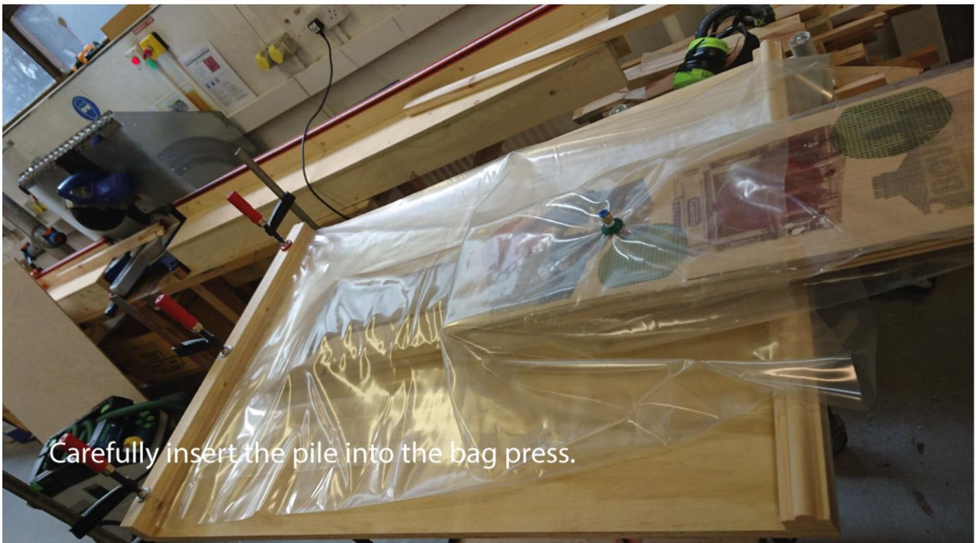
Carefully insert the pile into the bag press.
