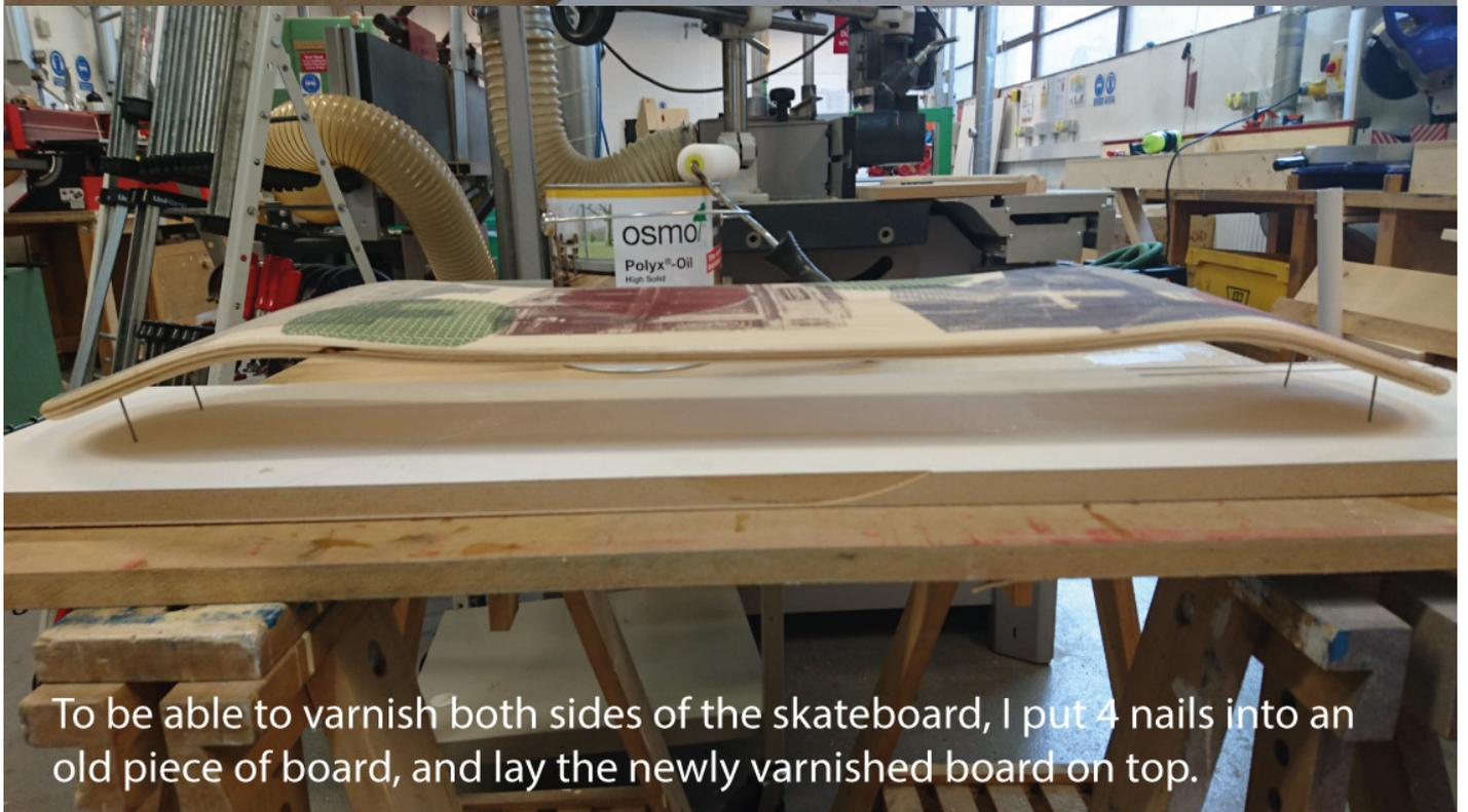
To be able to varnish both sides of the skateboard, I put 4 nails into an old piece of board, and lay the newly varnished board on top.
