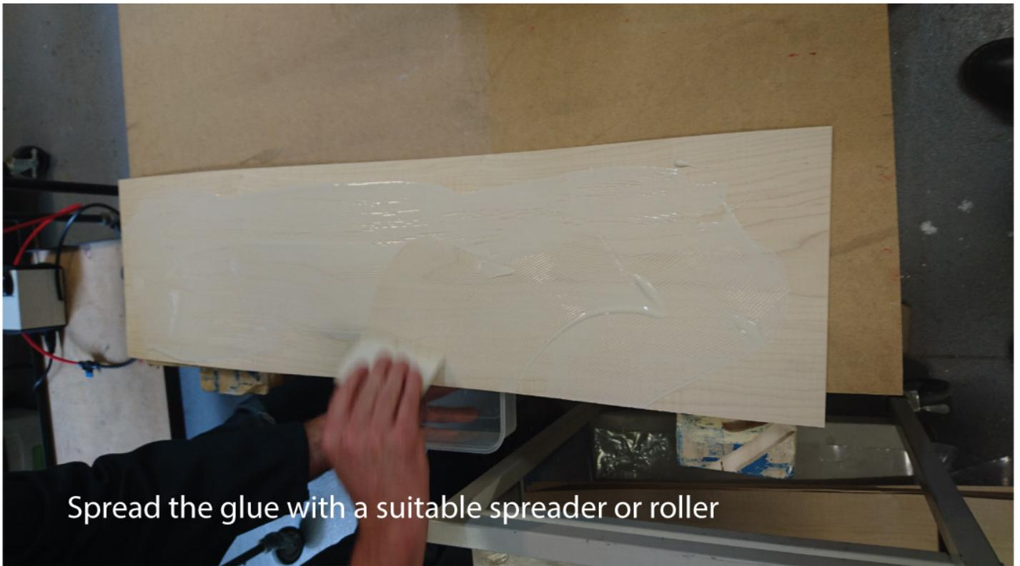
Spread the glue with a suitable spreader or roller
