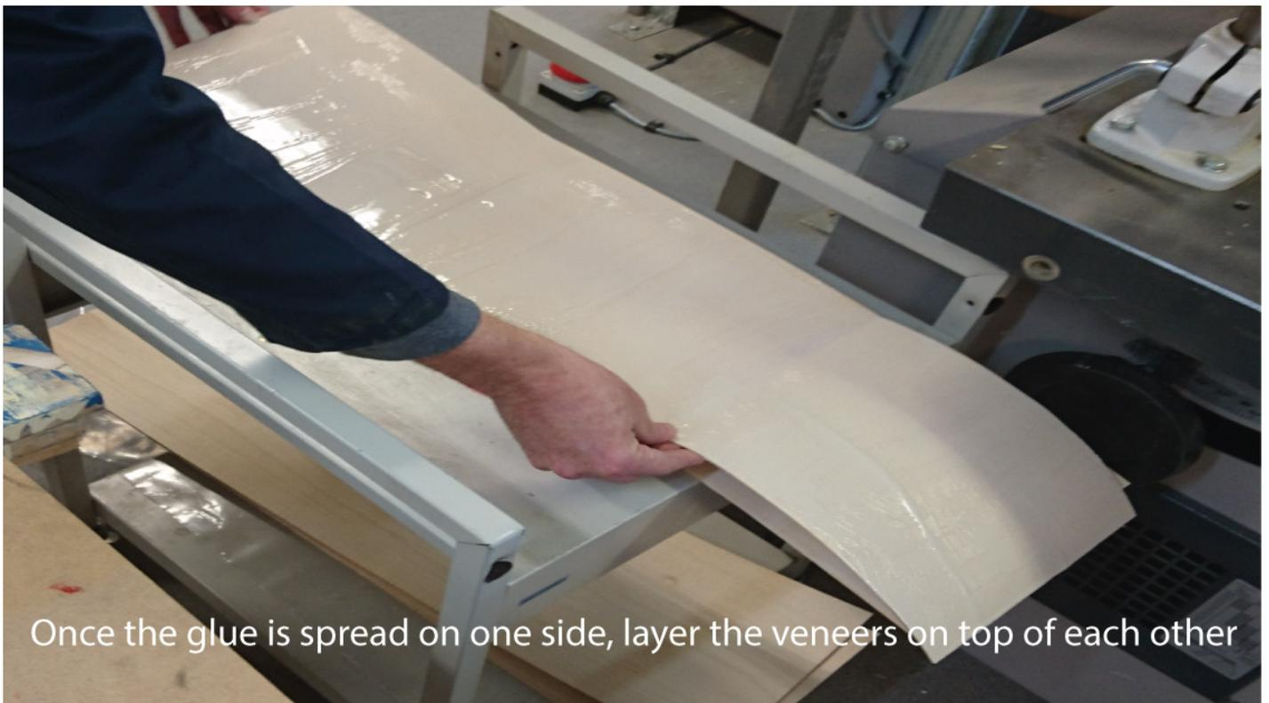
Once the glue is spread on one side, layer the veneers on top of each other
