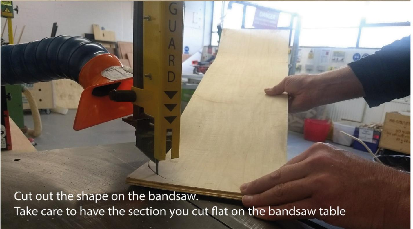
Cut out the shape on the bandsaw.
