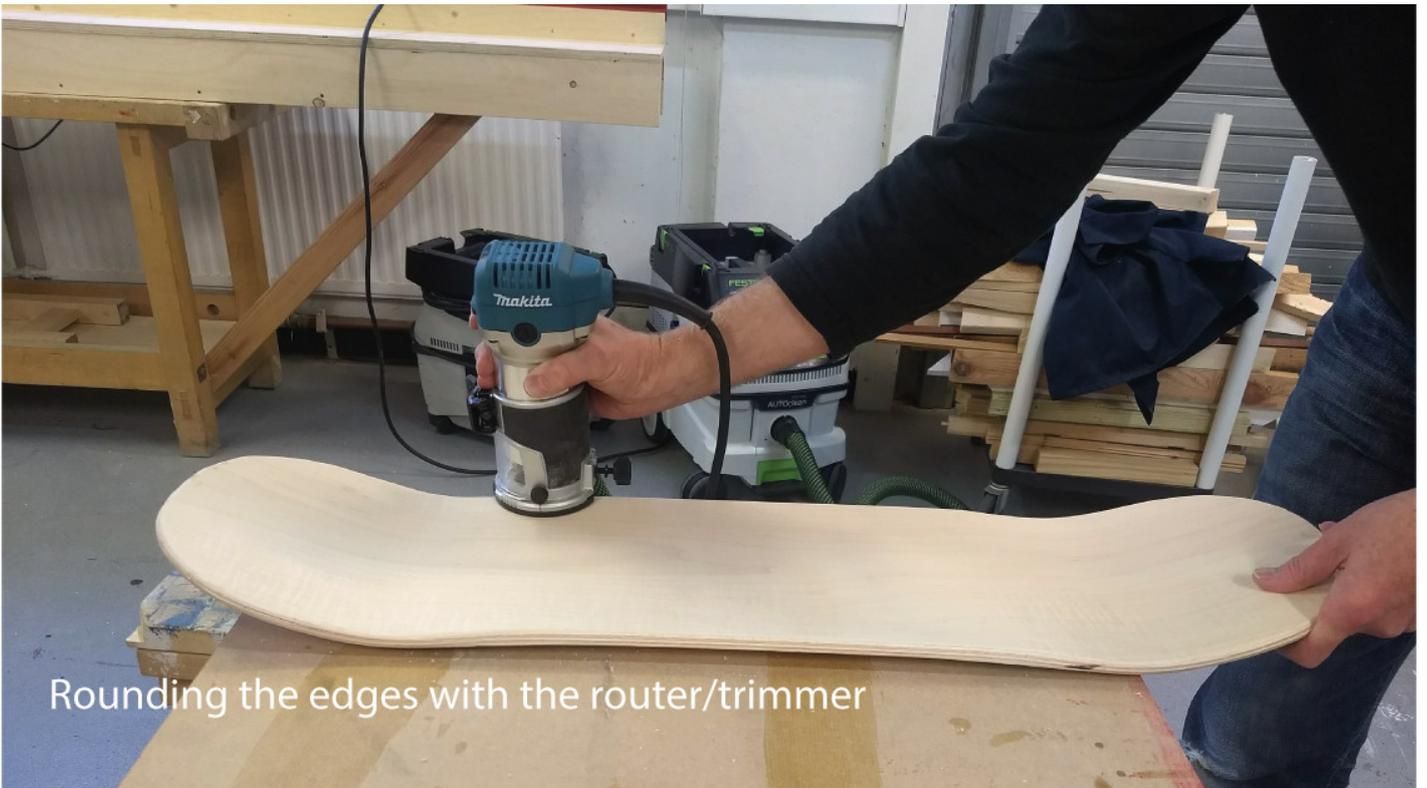
Rounding the edges with the router/trimmer
