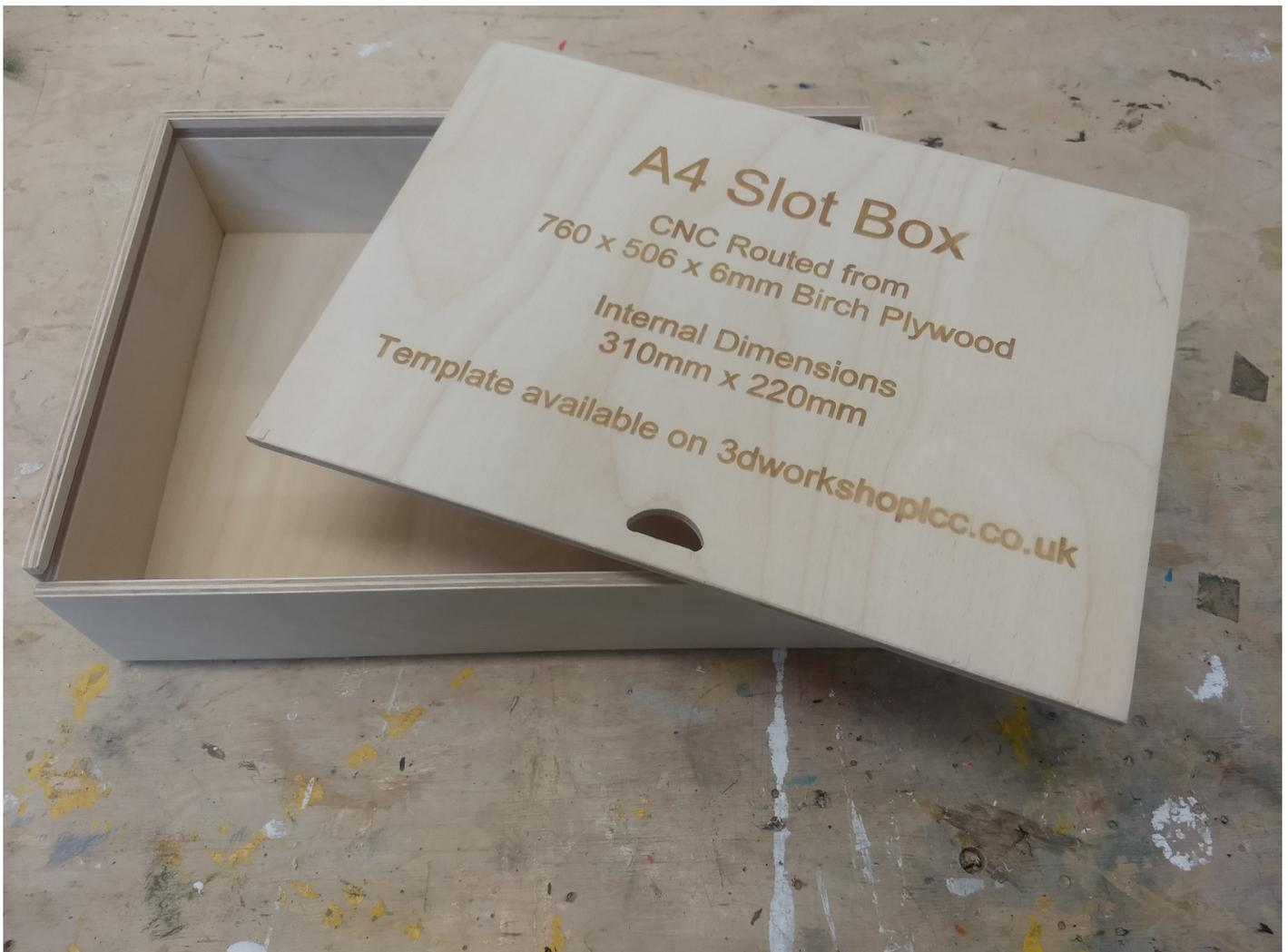
CNC routing is a quick and easy way to create a Slot Box. On the left you can download the files for A4 and A5 sized slot boxes like the one above. These files are for reference only. They have been prepared and programmed so that they can be run on the CNC Router.
