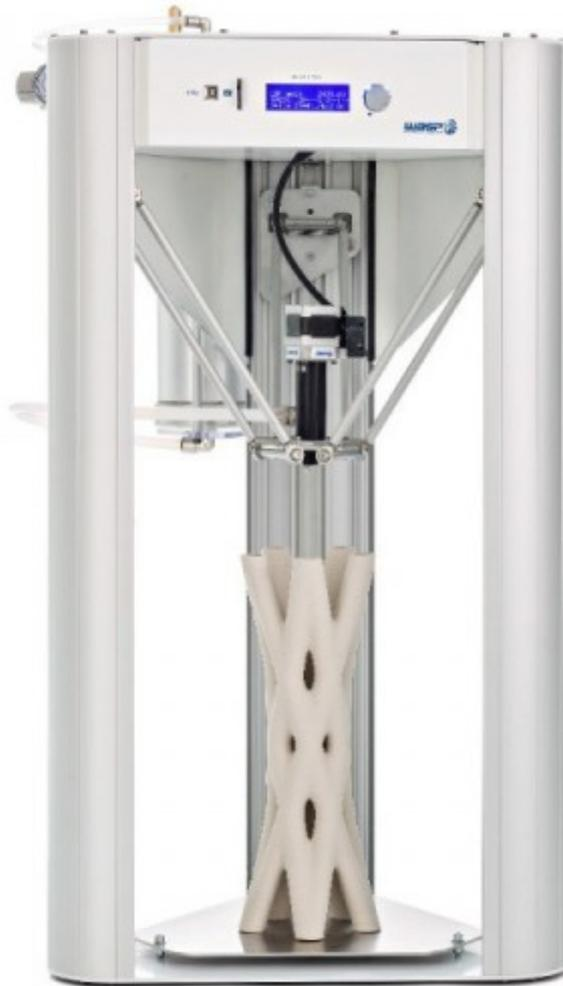
The Wasp Delta 3D printer is an experimental printer. You should expect to spend a significant amount of time printing. Unlike the other printers in the workshop you must stay with the machine while it is printing. This is because you need to adjust the settings during printing or it will fail. The Wasp is quicker than other printers and a medium sized print will usually take about 1 hour 30 minutes. You can pause the machine at any time.
