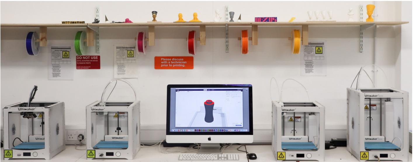
Ultimaker is a brand of 3D Printer which uses a technique known as [Fused Deposition Modelling](#) (FDM) or [Fused Filament Fabrication](#) (FFF). This technique uses a string of thermoplastic material (filament) which is pushed through a heated nozzle. The printer lays down melted material at a precise location, which then cools and solidifies, building the print layer-by-layer.
